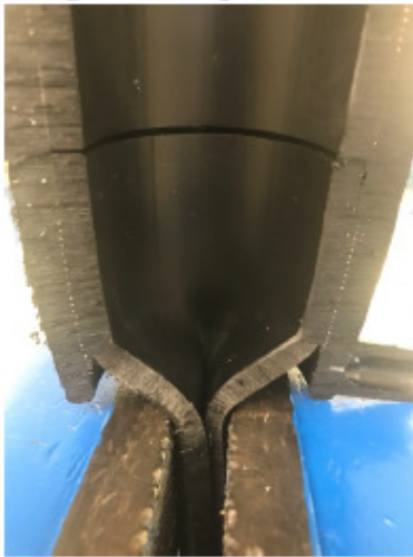
Coupling Crush Test - Passing Result
