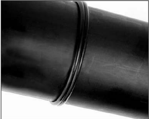
Figure 8.3 – Acceptable Visual Appearance (Reference ASTM F2620 X2)
