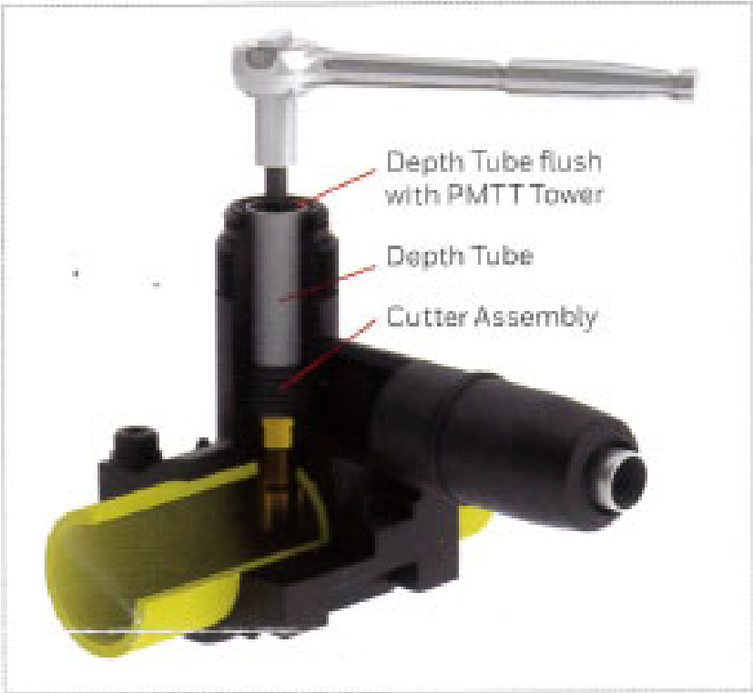
Fig. 4 - Full installation of Cutter Assembly, Cutter Sleeve engaged in (PE) Main, Depth Tube is flush with top of PMTT Tower
