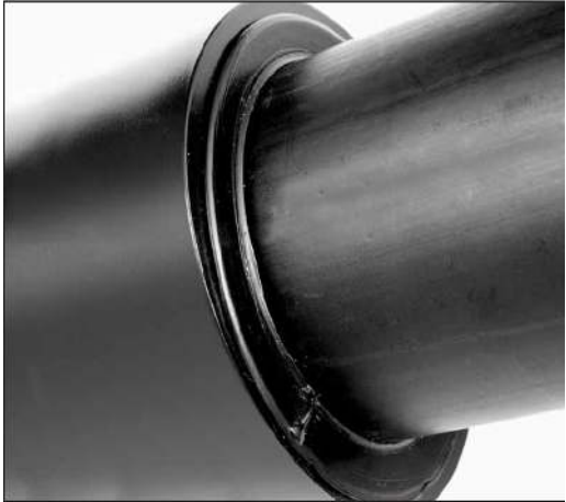
Figure 7.1 – Acceptable Visual Appearance (Reference ASTM F2620 X2)
