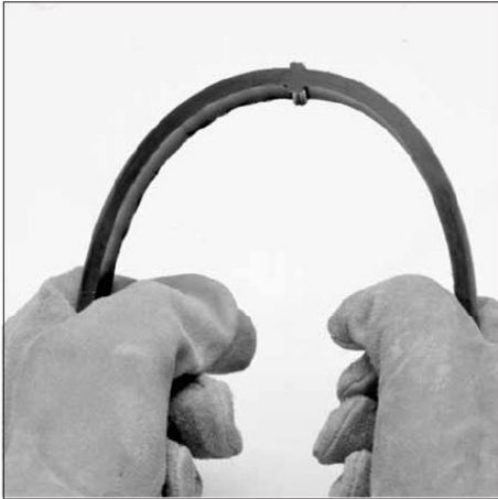
Figure 6.0a - Butt Fusion Qualification
