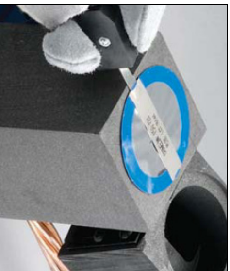
Figure 6. Attachment of electronic ignitor to charge
