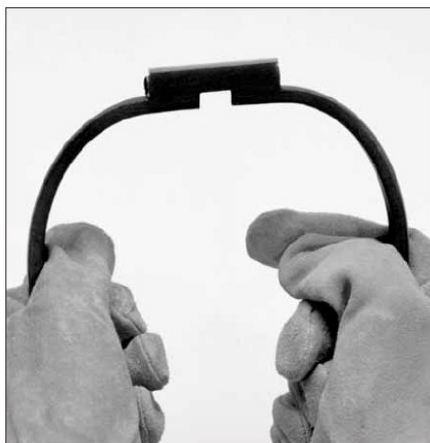
Figure 6.0a - Socket Fusion Qualification
