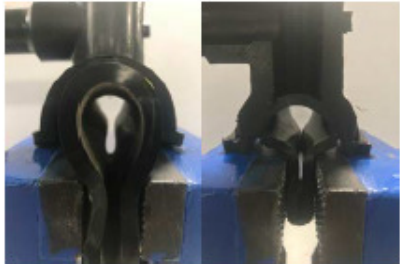
Saddle Crush Test – Passing Result
