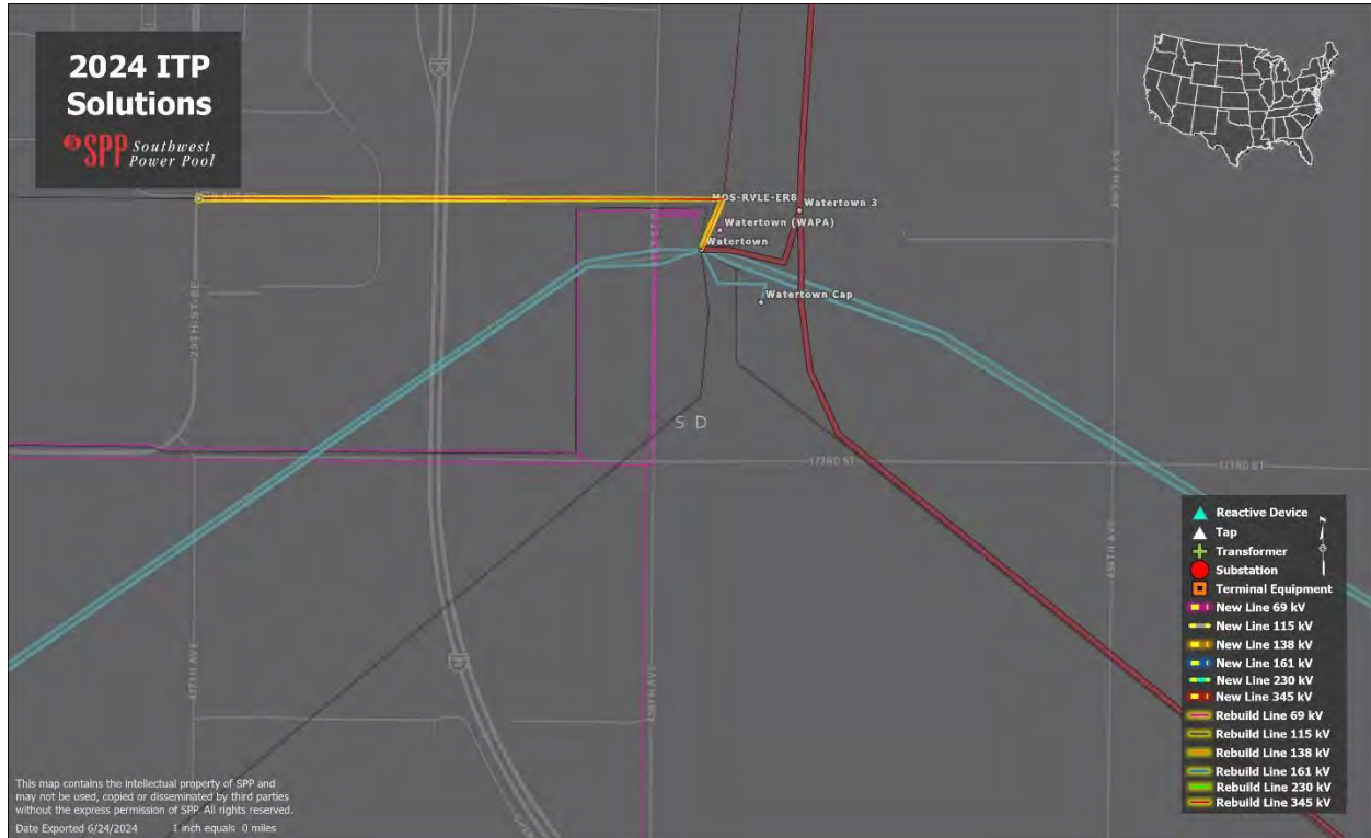
Figure 6.41: UMZ: 15th Ave – Watertown 115 kV Rebuild
