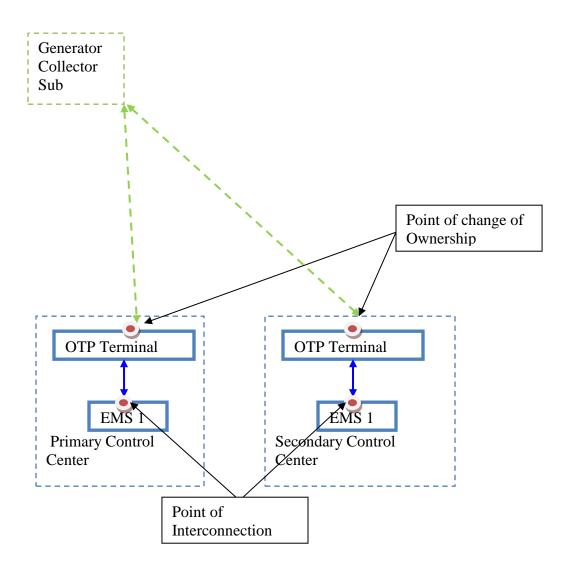
Exhibit A2–3 Transmission Owner Relay Protection One Line Diagram
