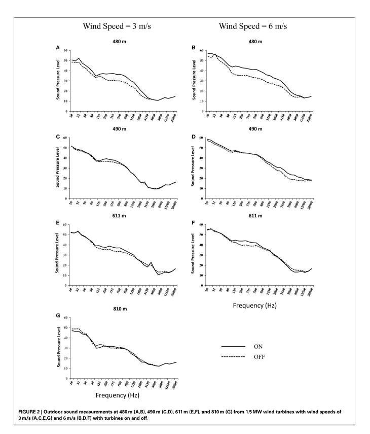
consistent. From these results, it is evident that during wind turbine operation, the increased sound levels that began in the LFN spectrum, at approximately 160 Hz and continued to 1000 Hz, were above auditory threshold levels and represented in the mean dB(A) sound measures. The consistency between the mean dB(A) measurements and trends observed in the 1/3-octave band analysis
