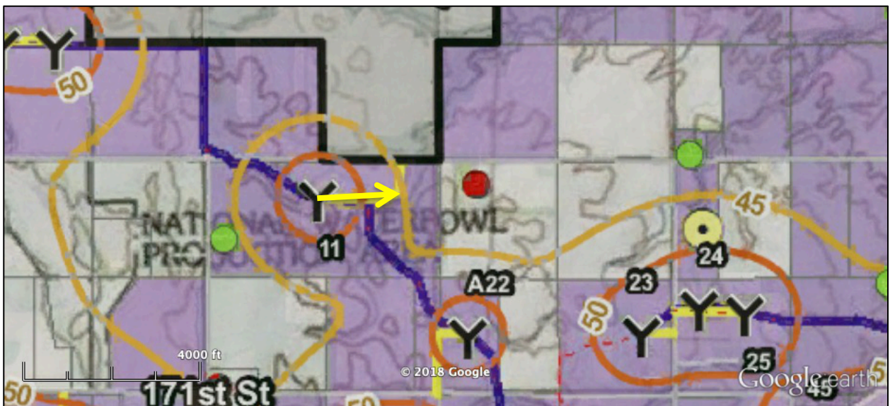
Figure 8.3 Predicted average noise levels including east of WT11, 50 and 45 dBA contours. Red dots are non-participating residences; green dots are participating. From November 2018 analysis. Yellow arrow shows analysis path.
