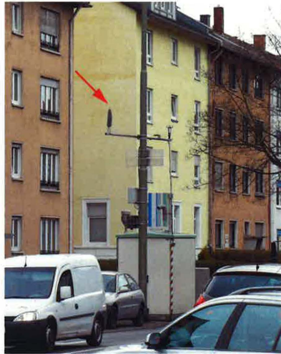
Figure 5.2-1: LUBW measuring station for detecting road traffic noise in Karlsruhe, Reinhold-Frank-Strasse. The arrow shows the location of the microphone. Residential buildings visible in the background. Photo: LUBW
