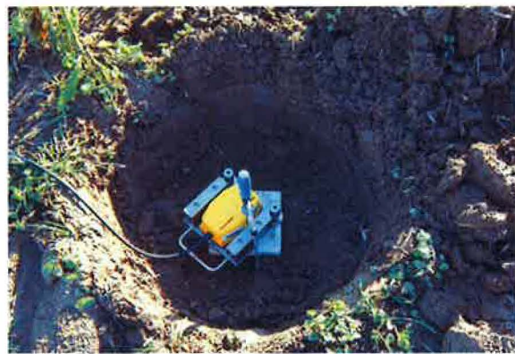
Figure 4.8-2: Vibration measurement point MP D on ground spike at a distance of 285 m from WT 5. Photo: Wölfel company
