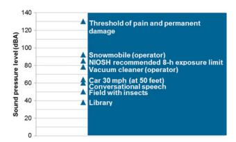
**FIGURE 2.** Sample A-weighted sound pressure levels.
