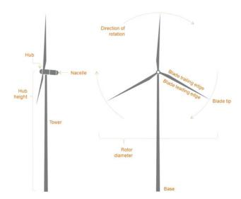
**FIGURE 1** . Schematic of a modern day wind turbine.
