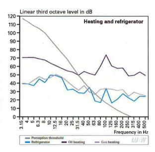
Figure 7.2-1: Third octave sound level of the noise from oil heating, gas heating and refrigerator at a distance of 0.5 m from the unit, with perception threshold according to Table A3-1 for comparison
