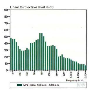
the infrasound levels between 2 Hz and 8 Hz are higher at night is unclear. The G-weighted level during the time elapsed was between 40 dB(G) at night and 65 dB(G) at day.
