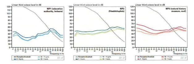
Figure 6-9: Comparative frequency-dependent representation of the third octave sound level for the three measurement points at different times of the day and at night. The results for MP2 and MP3 have been corrected (reverberant plate, see Section 4.1). The perception threshold was also shown as a means of orientation. Left: measurement point MP1 (education authority, indoors); Centre: measurement point MP2 (Friedrichsplatz); right: measurement point MP3 (natural history museum, roof).
