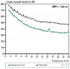
Figure 4.3-2 Narrow band spectra of background noise and total noise in the vicinity of the wind turbine WT 2 for the frequency range of infrasound
