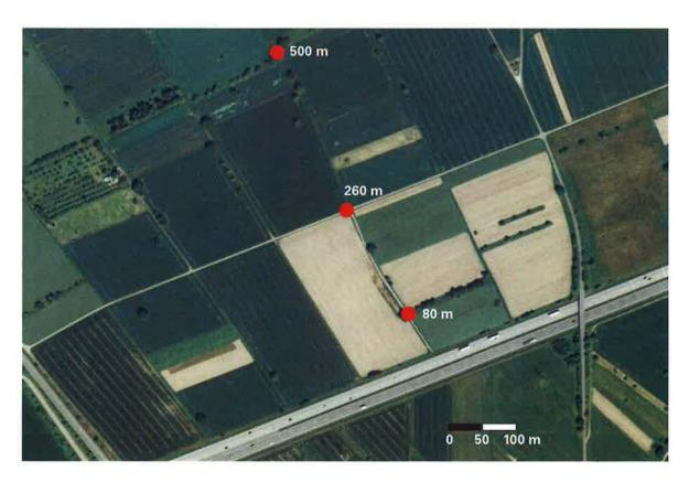
Figure 5.3-1: Location of the measurement points at the A5 motorway south of Karlsruhe near Malsch, indicating the distances between the microphone positions and the centre of the motorway. The town of Malsch is located outside of the picture at the bottom left. The B3 main road is located above the picture. Picture source: LUBW, LGL
