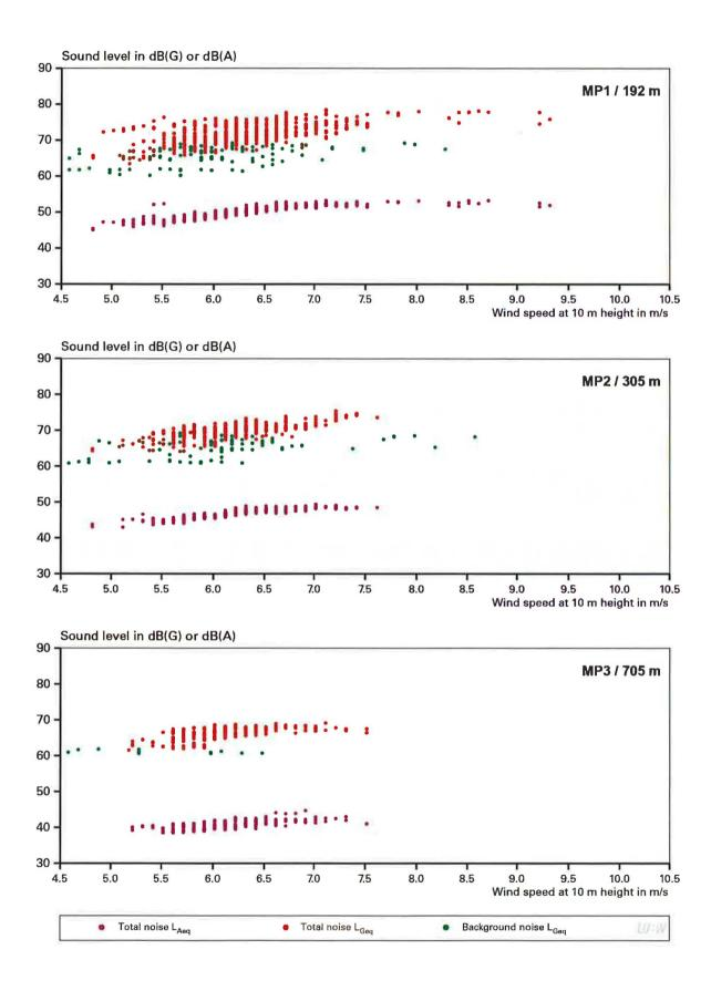
Figure 4.7-6: Audible sound level (A level) and infrasound level (G level) depending on the wind speed for the wind turbine WT 6. The G levels when the turbine is switched on (red dots) and when the turbine is switched off (green dots) are shown, as are the A levels with the turbine switched on (violet dots).
