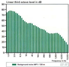
Figure 4.3-3: Third octave spectra of total noise and background noise in the vicinity of the wind turbine WT 2
