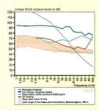
Comparison of noise levels within a passenger car, near a road, on an open field, and from an od heating with the level range of the measured wind turbines as well as the human perception threshold.
