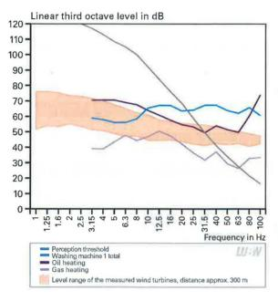
Firgure 2-4: Comparison of noise of technical appliances in residential buildings with the level range of wind turbines at a distance of approx, 300 m as well as the perception threshold according to Table A3-1 regarding infrasound and low-frequency noise. For measuring corrections, see Section 4.1.
