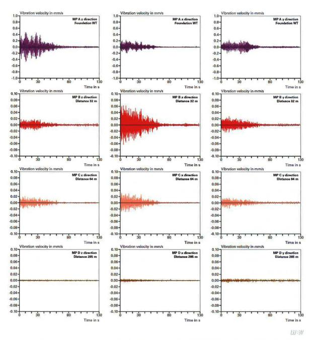
**Figure 4.8-4**: Representation of the decreasing vibration after shutdown of the wind turbine 5 for all measurement points and directions. From top to bottom: Measurement points MP A to MP D; left to right: Spatial directions z, x and y. The shutdown of the turbine followed at 12:32 p.m. – Note the different scale of the vibration velocity at the measurement point MP A (foundation, top row).
