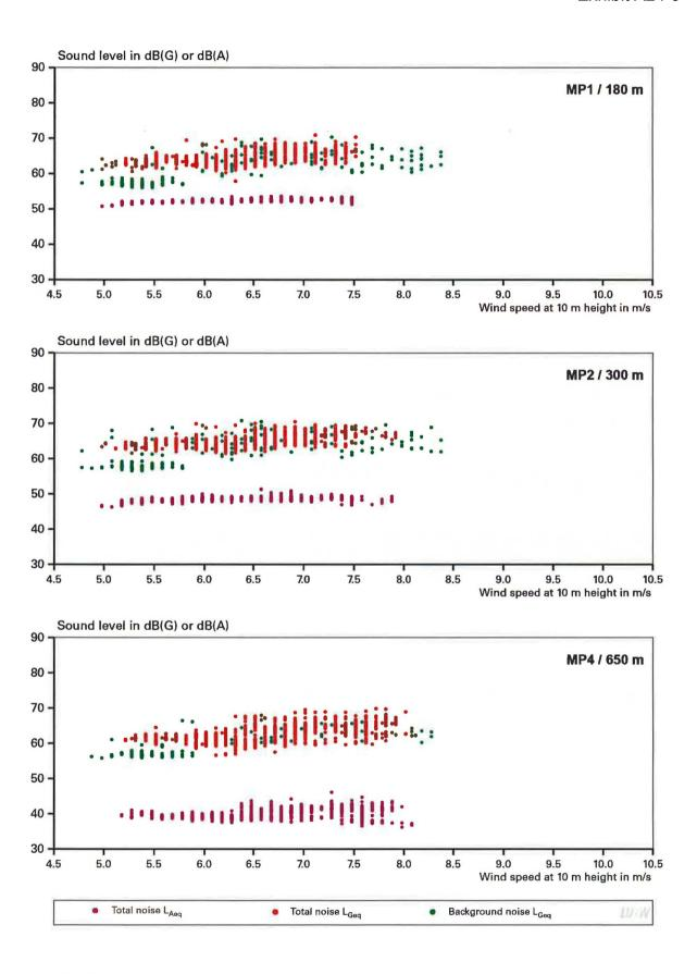
Figure 4.5-12: Audible sound level (A level) and infrasound level (G level) depending on the wind speed for the wind turbine WT 4. The G levels when the turbine is switched on (red dots) and when the turbine is switched off (green dots) are shown, as are the A levels with the turbine switched on (violet dots).
