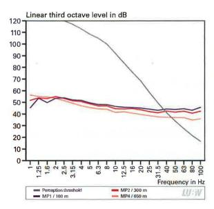
Figure 4.5-11: Third octave spectra of total noise at the measurement points MP1 (180 m), MP2 (300 m) and MP4 (650 m) of WT 4, with the perception threshold according to Table A3-1 in comparison. The measured values were corrected according to Section 4.1.
