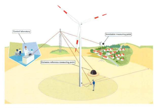
Figure 9.2-1: Basic design of a possible long-term monitoring station
