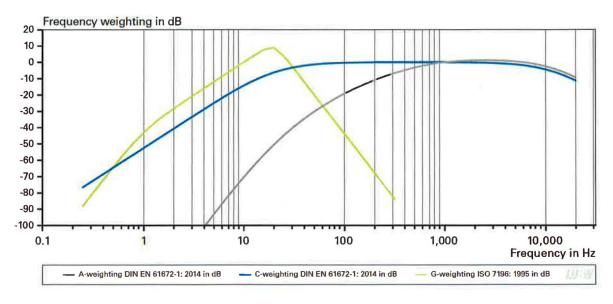
Figure A3-1: Course of the frequency weighting curves A, C and G in the range below 500 Hz according to ISO 7196 and DIN EN 61672-1 (2013) [22]
