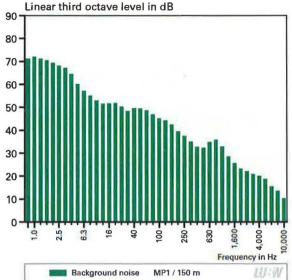
Figure 4.2-4: Third octave spectra of total noise and background noise in the vicinity of the wind turbine WT 1
