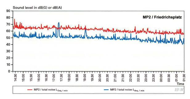
Figure 6-10: Course of the A and G-weighted sum level  $L_{Aeg}(t)$  und  $L_{Geq}(t)$  at the measurement point MP2 (Friedrichsplatz) in the time period 20,09,2013, approx. 2:30 p.m. to 21.09.2013, 1:30 a.m.
