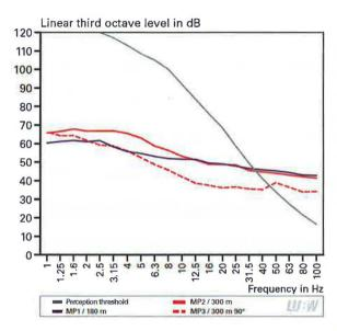
Figure 4.4-5: Third octave spectra of the total noise at the measurement points MP1 (180 m), MP2 (300 m) and MP3 (300 m, offset by 90 °) of wind turbine 3, perception threshold according to Table A3-1 for comparison. The measured values were corrected according to Section 4.1.
