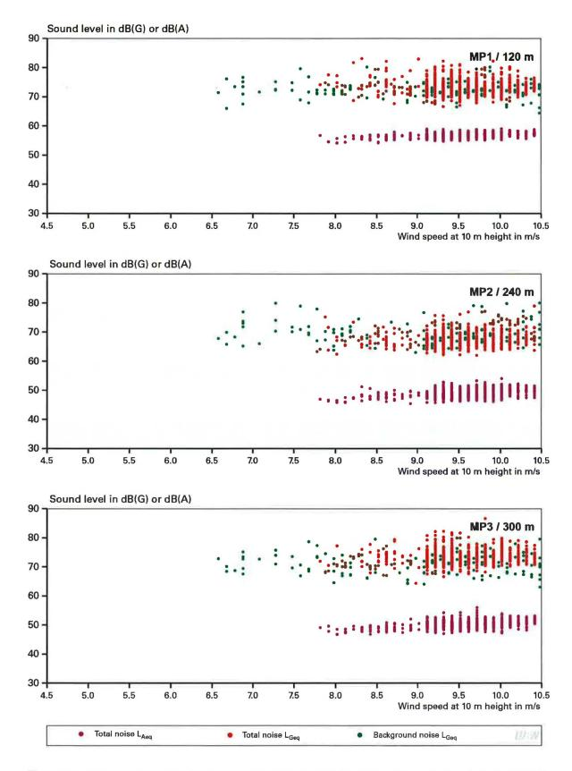
**Figure 4.3-5**: Audible sound level (A level) and infrasound level (G level) depending on the wind speed for the wind turbine WT 2. The G levels when the turbine is switched on (red dots) and when the turbine is switched off (green dots) are shown, as are the A levels with the turbine switched on (violet dots).
