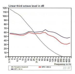
Firgure 5.3-2: Frequency-dependent representation (linear third octave level) of a measurement at the motorway A5. As a comparison, the perception threshold according to Table A3-1 was also included. Note: The representation begins at a frequency of 3.15 Hz (in other illustrations partly from 1 Hz or 6.3 Hz). This is due to the measuring technology used.
