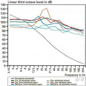
Firgure 5.4: Low-frequency sound (averaging level) in the inside of car and minibus driving at approx. 130 km/h in comparison to the perception threshold according to Table A3-1
