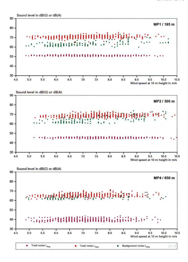
Figure 4.6-8: Audible sound level (A level) and infrasound level (G level) depending on the wind speed for the wind turbine WT 5. The G levels when the turbine is switched on (red dots) and when the turbine is switched off (green dots) are shown, as are the A levels with the turbine switched on (violet dots).
