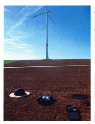
Figure 4.5-1 (right): Measurement points MP2 and MP3 at a distance of 300 m from the tower axis. Reverberant plate and double wind screen (left), spanned hole in the ground (right). Photo: Wölfel company
