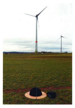
Figure 4.7-1: Wind turbine WT 6 in surroundings used for agricultural purposes. The measurement point MP1 with reverberant plate and dual wind screen can be seen in the foreground. Photo: Wölfel company
