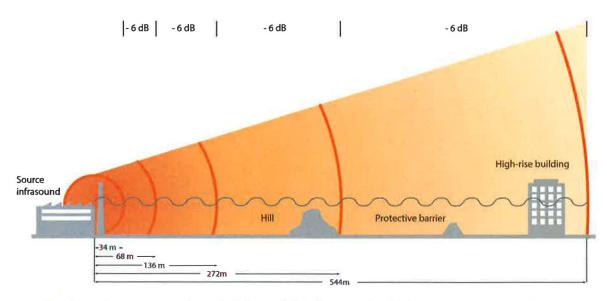
Figure A1-1: Exemplary presentation of spread of infrasound with a frequency of 10 Hz. The associated wavelength of 34 m is larger than the height of houses, trees and protective barriers. Therefore these hardly absorb the sound. However, the sound pressure level nevertheless decreases according to the same law as for audible sound: Each doubling of distance from the source results in a decrease in sound level of 6 dB. Image source: Bayerisches Landesamt für Umwelt [15]
