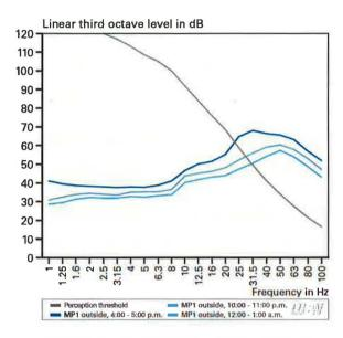
Figure 5.1-4: Comparison of the corrected linear third octave levels, determined at the measurement point MP1 (outside the building) for the averaging periods 4:00 - 5:00 p.m., 10:00 - 11:00 p.m., and 12:00 - 1:00 a.m. Furthermore, the perception threshold is also shown (see Section 4.1).
