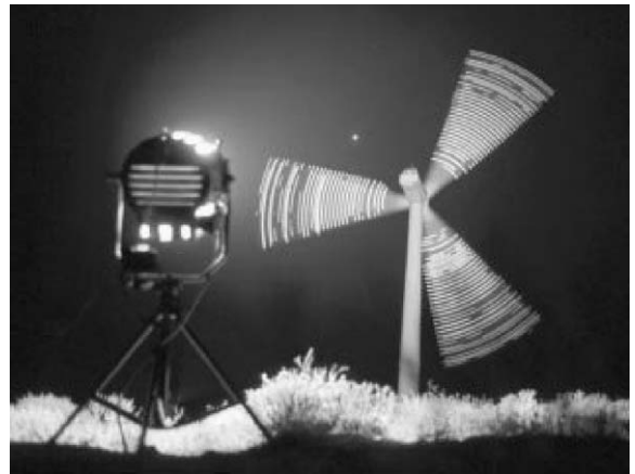
Fig. 13. Recording of stall-flag signals from the NEG Micon turbine in California (from [32], © Nature, with permission).
