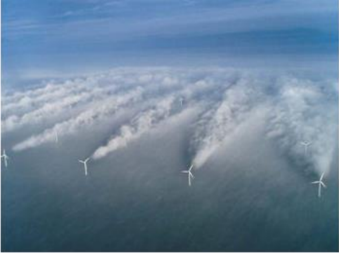
Figure 2: Turbulence effects from wind turbines.
