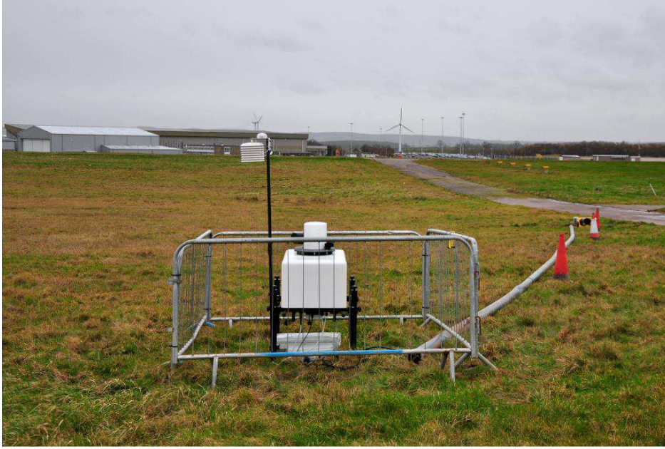
Figure 3.9: The on-site Galion LIDAR.
