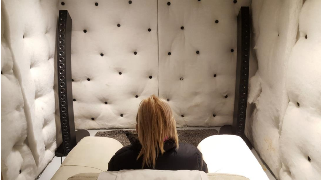
Figure 12: TAG hemi-anechoic room with line array speakers
