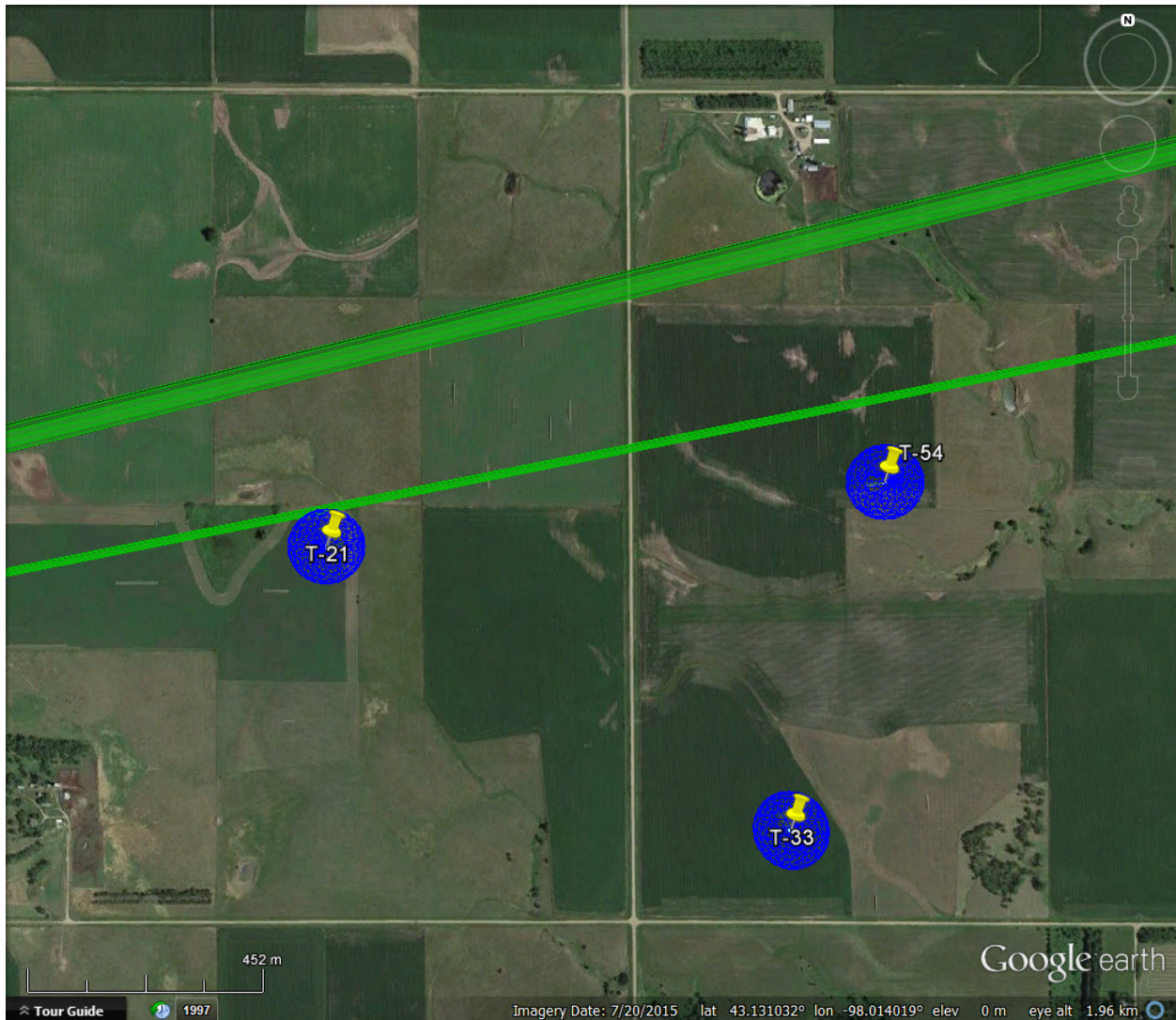
Figure 5 – Turbines 21 and 54 Close to Microwave Path WNER900/WQRU421
