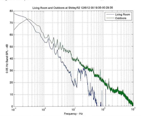
Measurements at the other residences R1 and R3 do not show this same result because the increased distance reduced periodic turbine noise closer to the background and/or turbine loads at the time of these measurements resulted in reduced acoustical emission. Future testing should be sufficiently extensive to cover overlapping turbine conditions to determine the decay rate with distance for this ultra low frequency range, or the magnitude of measurable wind turbine noise with distance.
