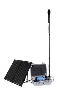
The dimensions of the case are approximately 2 feet by 1.5 feet by 0.5 feet. The solar panel is approximately 2 feet by 3 feet. Tripods and/or metal T-posts (driven by hand 1 to 2 feet into the ground) may also be used. The testing period will last two to four weeks and will require periodic access (approximately one hour each) for technicians to check on the equipment. The specific timing is expected to be finalized this month.
