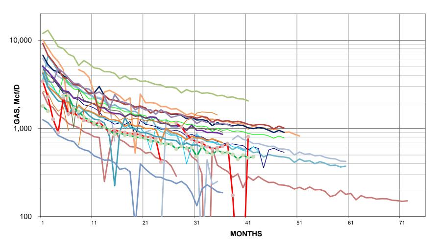
Note: Each line represents daily production from one well over time. Sharp, short-term decreases represent periods a well was temporarily either not producing or producing at a reduced rate until the triggering production issue could be remedied.
