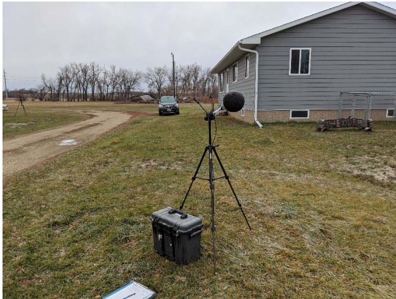
Figure 6-4 Location 3 - Photo of Sound Level Measurement Location (Pickup)
