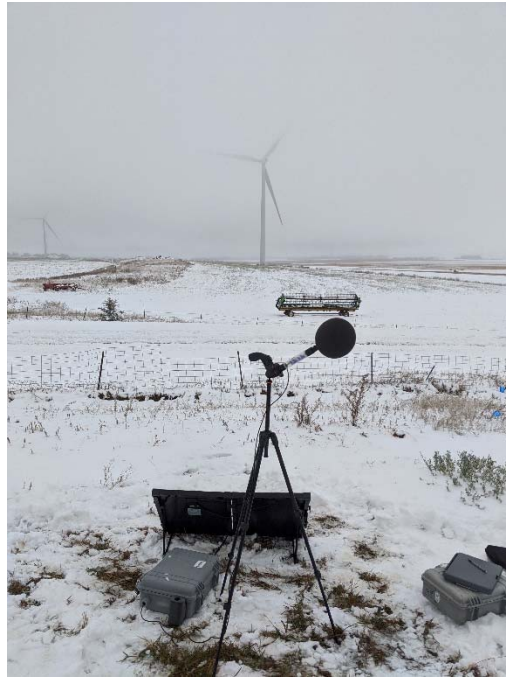
Figure 6-2 Location 1 - Photo of Sound Level Measurement Location (Setup)
