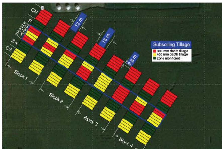
FIGURE 3 Based on the randomized complete block design (RCBD), the 300-mm- and 450-mm-deep tillage treatments were applied within Zone-1, Zone-2 and Zone-3 prior to topsoil replacement (“blue” rectangle). Each subsoil tillage plot size was 7.6 m width by 18 m long. Within the right-of-way (ROW), Zone-x and Zone-P (topsoil pile zone) were not part of the RCBD tillage experiment design. Crop field zones (Control-N, CN (north) and Control-S, CS (south)) were outside the ROW and unaffected by the pipeline construction [Colour figure can be viewed at wileyonlinelibrary.com ]
