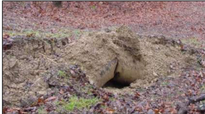
Figure 6-2. A severe buckle formed at zero internal pressure
