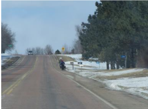
Four foot wide shoulder (Six Mile Rd.) - Accommodates all transportation and recreation modes on a minor arterial with a relatively low posted speed limit
