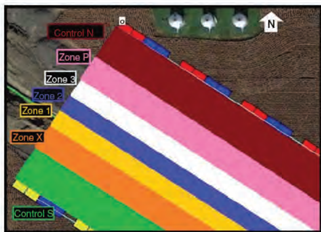
FIGURE 2 Map of experimental research plot showing the designated construction zones (Zone-1, Zone-2, Zone-3 and Zone-x) and unaffected crop field zones (Control-S and Control-N) aligned in reference to the pipeline. Zone-P refers to where the topsoil was piled. Colour figure can be viewed at wileyonlinelibrary.com
