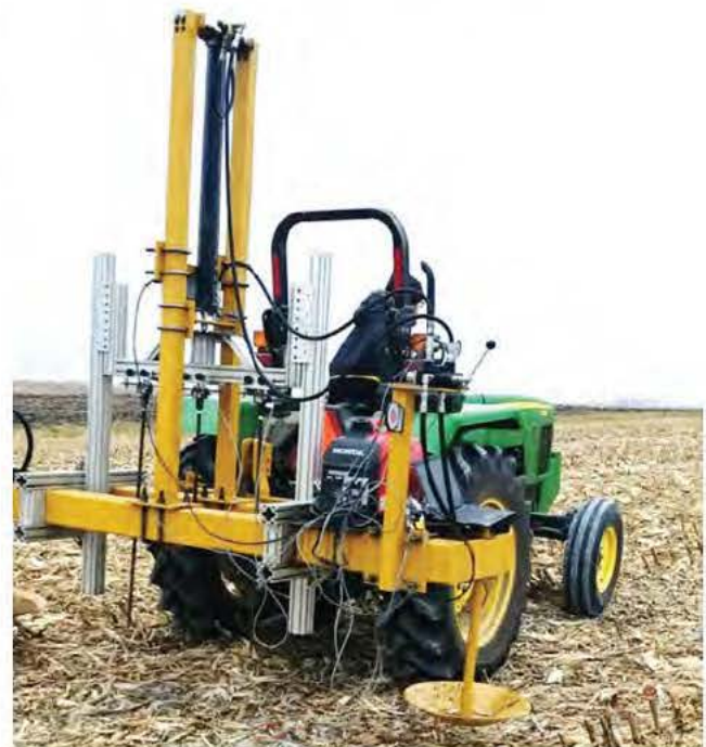
FIGURE 4 Three-probe cone penetrometer mounted on the three-point hitch of a tractor. The lateral spacing between the penetrometer probes was 150 mm during field measurements. An ASABE 30-degree conical tip with 285 mm 2 cone base area was attached to each of the probes. The probe insertion rate was 30 mm s -1 [Colour figure can be viewed at wileyonlinelibrary.com ]
