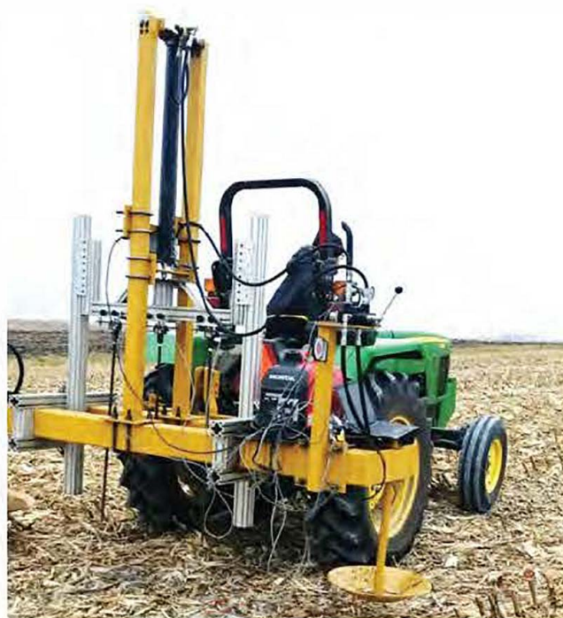
FIGURE 4 Three-probe cone penetrometer mounted on the three-point hitch of a tractor. The lateral spacing between the penetrometer probes was 150 mm during field measurements. An ASABE 30-degree conical tip with 285 mm 2 cone base area was attached to each of the probes. The probe insertion rate was 30 mm s -1 [Colour figure can be viewed at wileyonlinelibrary.com ]
