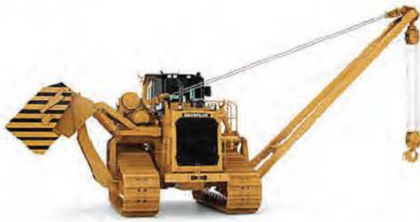
Caterpillar pipe liner PL 87. Fully loaded weight = 475 kN. Each track dimension had a nominal track contact length, which is the length of track in contact with a flat, unyielding surface (ISTVS, 1977), of 3.71 m and a width of 0.76 m.
