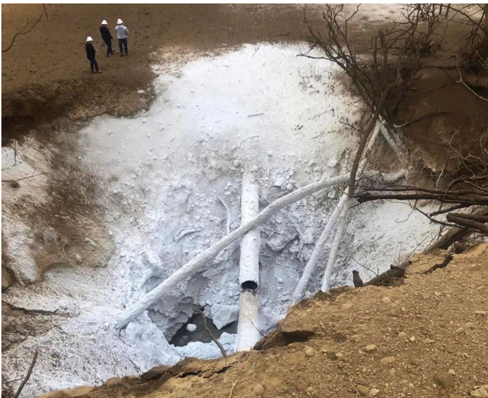
LEFT: The CO2 pipeline rupture. RIGHT: Vehicles pass over the pipeline explosion site in Satartia in July. Yazoo County Emergency Management Agency/Rory Doyle for HuffPost
