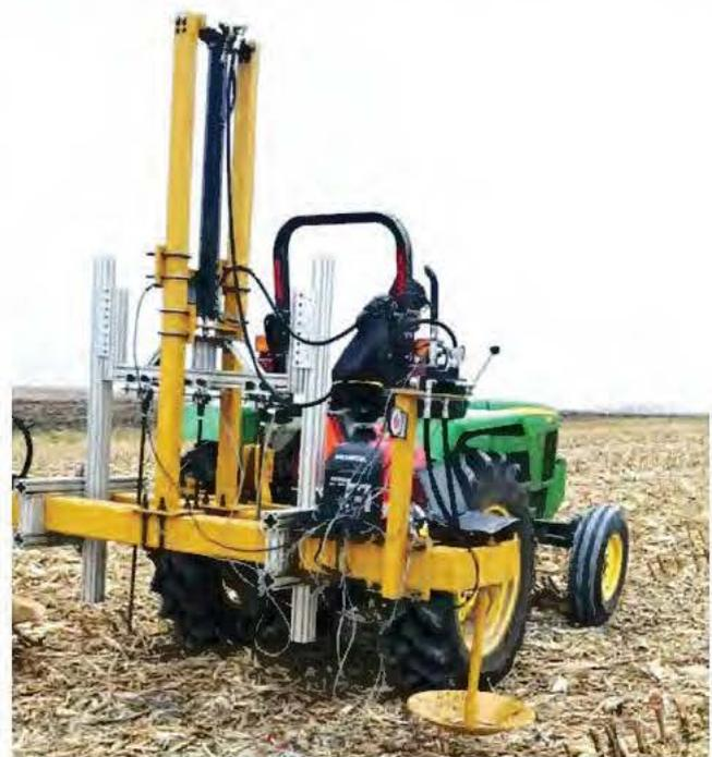
**FIGURE 4** Three-probe cone penetrometer mounted on the three-point hitch of a tractor. The lateral spacing between the penetrometer probes was 150 mm during field measurements. An ASABE 30-degree conical tip with 285 mm<sup>2</sup> cone base area was attached to each of the probes. The probe insertion rate was 30 mm s<sup>-1</sup> [Colour figure can be viewed at [wileyonlinelibrary.com](http://wileyonlinelibrary.com)]
