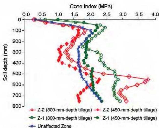
**FIGURE 8** Soil cone index profile measured from the right-of-way (ROW) zones (Zone-1 and Zone-2) subsoiled at 300-mm- and 450-mm-depth tillage treatments prior to the topsoil replacement and the unaffected zone outside the ROW. The topsoil depth refers to the topsoil surface from the unaffected zone. Each data point is a mean of four replicates of the three-point cone penetrometer readings [Colour figure can be viewed at [wileyonlinelibrary.com](http://wileyonlinelibrary.com)]
