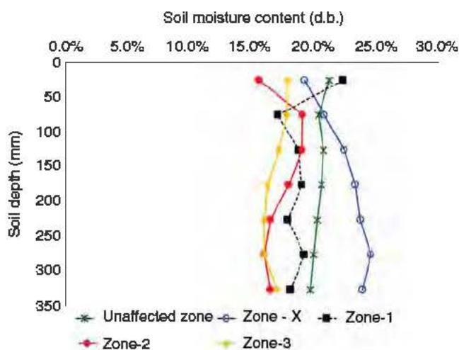
**FIGURE 7** Soil moisture content of soil depth from four construction zones Zone-1, Zone-2, Zone-3, Zone-x and an unaffected zone (Control-S). The reported soil depth refers to the top surface of the exposed subsoil within the ROW. Each data point is a mean of nine replicates [Colour figure can be viewed at [wileyonlinelibrary.com](http://wileyonlinelibrary.com)]
