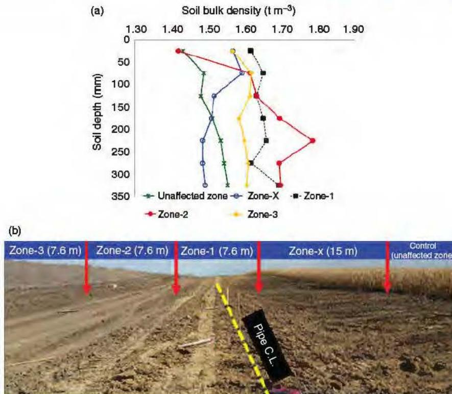
**FIGURE 6** Soil bulk density with depth from the construction ROW zones (Zone-1, Zone-2, Zone-3 and Zone-x) and the unaffected zone (Control-S). The reported soil depth refers to the top surface of the exposed subsoil (b) within the ROW. “C.L.” is the pipe centreline. Each data point is a mean of nine replicates [Colour figure can be viewed at [wileyonlinelibrary.com](http://wileyonlinelibrary.com)]
