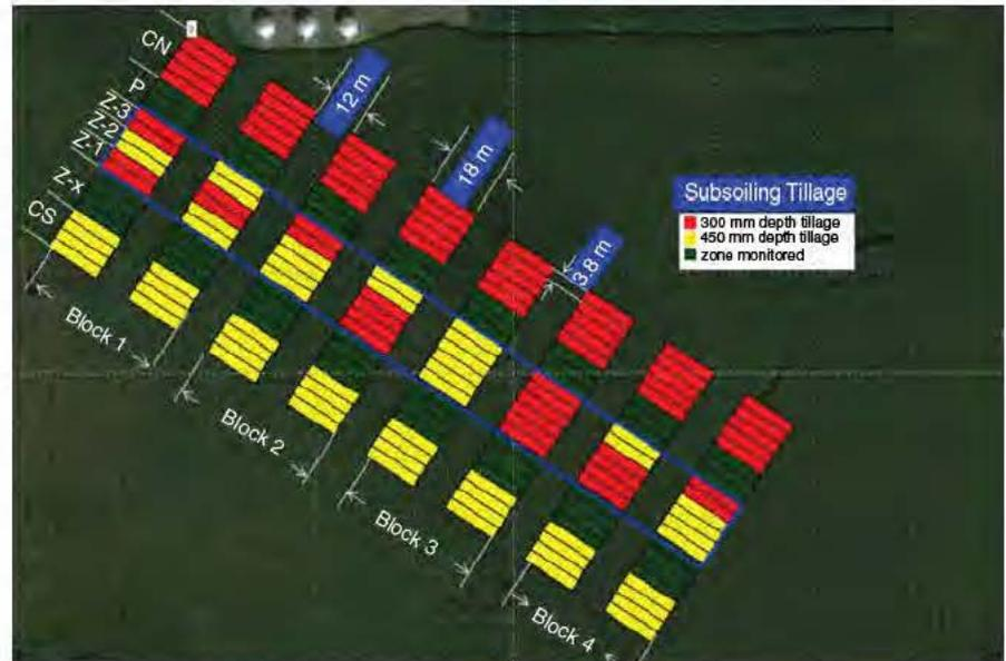
760 mm spacing with DMI ripper points, 63.5-mm-wing width) was used to apply the subsoil tillage operation.
