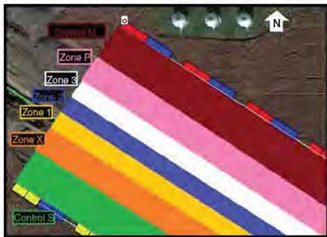
**FIGURE 2** Map of experimental research plot showing the designated construction zones (Zone-1, Zone-2, Zone-3 and Zone-x) and unaffected crop field zones (Control-S and Control-N) aligned in reference to the pipeline. Zone-P refers to where the topsoil was piled
