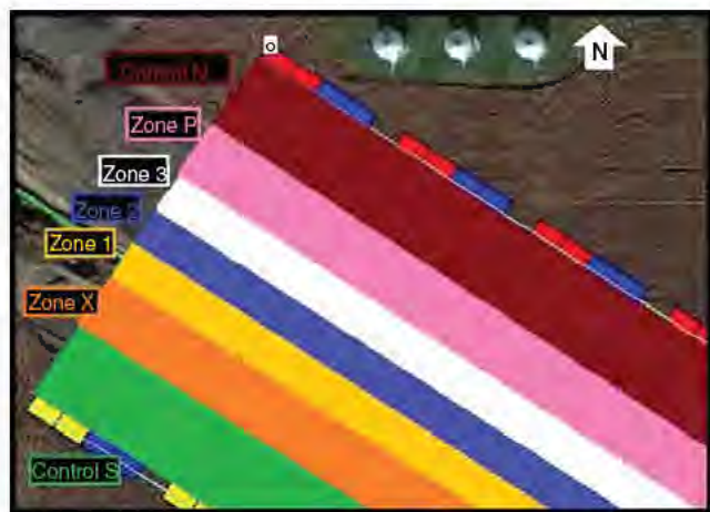
FIGURE 2 Map of experimental research plot showing the designated construction zones (Zone-1, Zone-2, Zone-3 and Zone-x) and unaffected crop field zones (Control-S and Control-N) aligned in reference to the pipeline. Zone-P refers to where the topsoil was piled Colour figure can be viewed at wileyonlinelibrary.com
