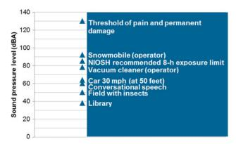
**FIGURE 2.** Sample A-weighted sound pressure levels.
