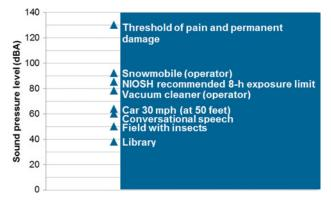
FIGURE 2. Sample A-weighted sound pressure levels.
