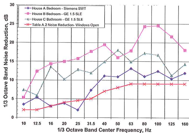
Fig. 20—One-third octave band interior noise reduction—Windows open.
