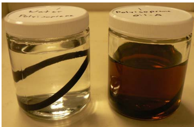
Figure 3.7. On the left is a polyisoprene gasket in de-chlorinated water and on the right is a polyisoprene gasket in Oil-A.
