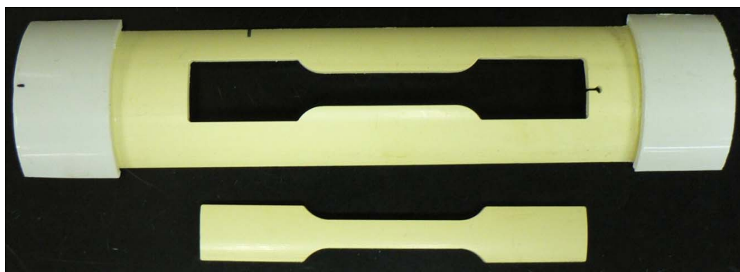
Figure 3.13. A dogbone is cut out of each 1/3 section of pipe to be tensile tested.
