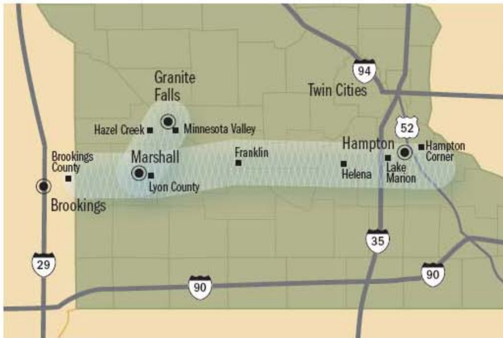
Figure 1 Proposed 345 kV line from White, SD Area to the Twin Cities Area
