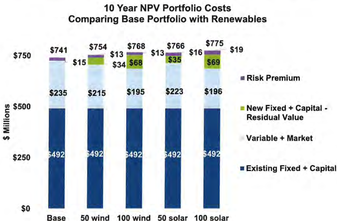
Figure 6-1 10-Year Net Present Value of Portfolio Costs, 2017-2026 (2017 $) Base, 50 MW wind, 100 MW wind, 50 MW solar, and 100 MW solar cases
