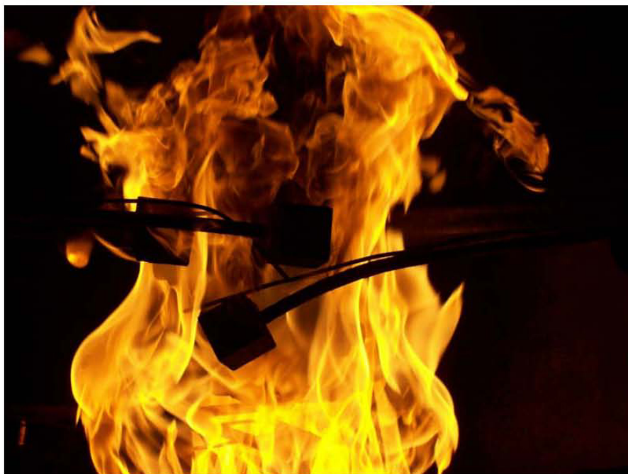
Figure 3 - Gasket Fire Test
