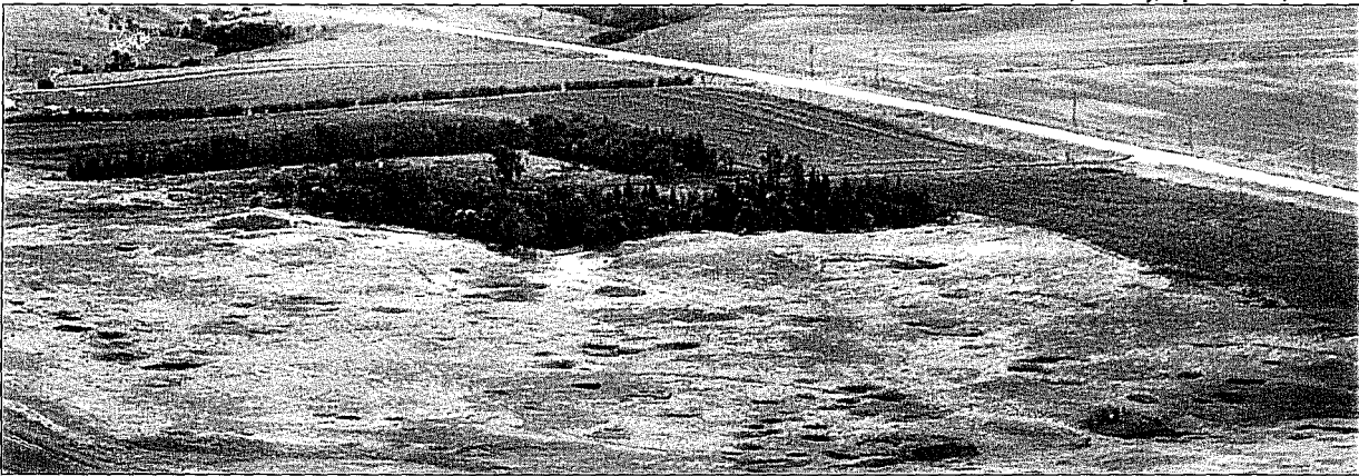
Before the second round of mining started, the Figenskau Mine area showed the signs of many sink holes caused by collapsing mine tunnels. Falkirk Mine chose to mine the site and reclaim the area so it could once again become a useful property. SUBMITTED
