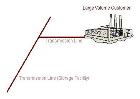
A pipeline that transports gas from a storage facility to a large volume customer is a transmission line.
