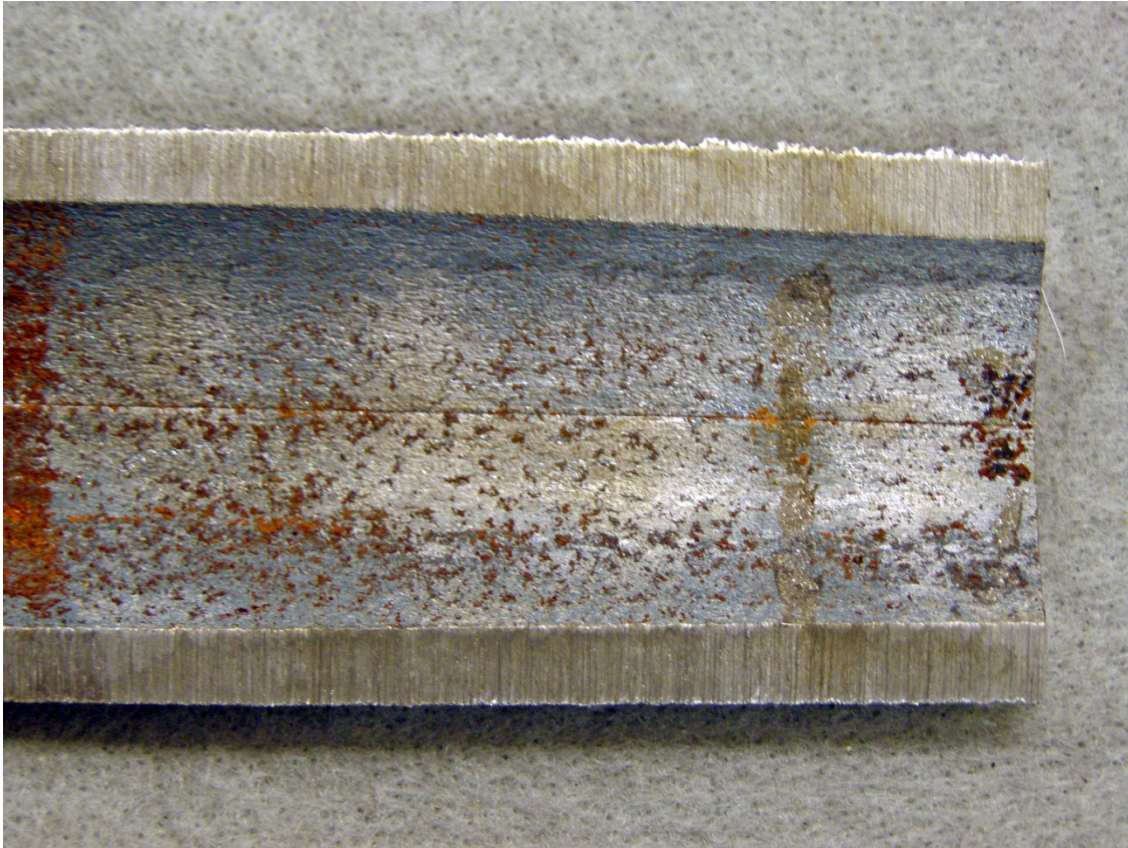
Figure 16. Score mark visible at ID surface that corresponded to butt-welded seam
