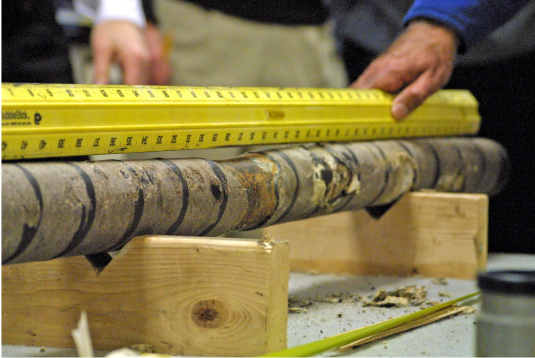
Figure 13. Deviation from straightness looking toward End A
