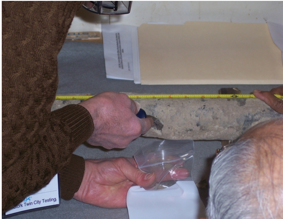
Figure 5. Illustration of sampling of coating and deposits that was done at eight locations along the pipe
