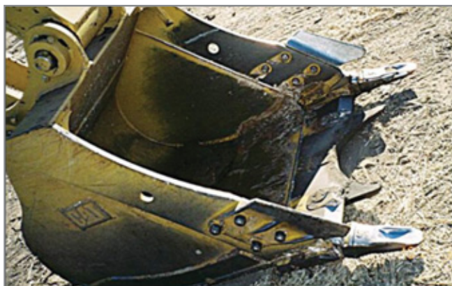
Half-moon spoon used to evacuate and conform 16" pipe.
