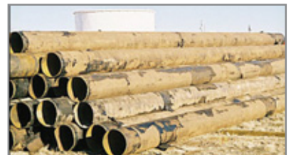
Coated pipe prior to cleaning.
