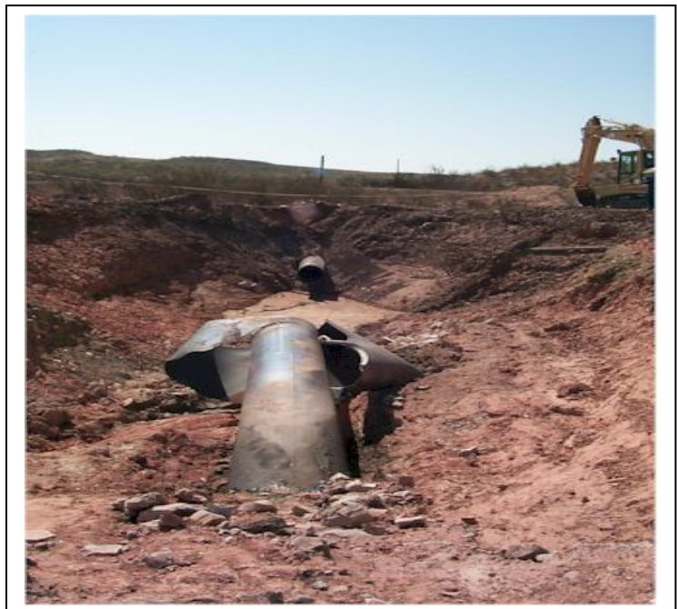
El Paso steel pipe that failed due to corrosion from inside the bottom of the pipeline.
