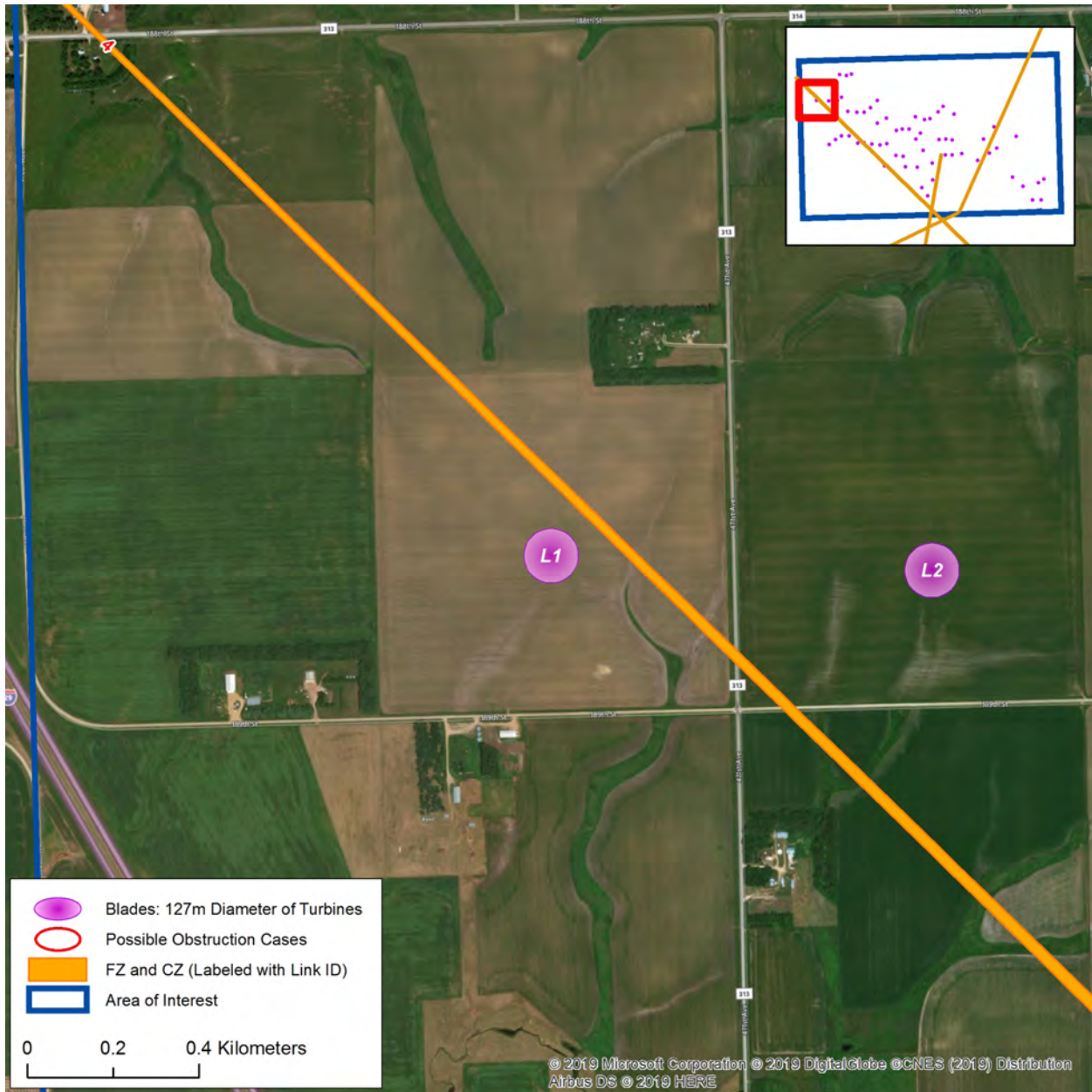
Figure 4: Microwave Paths with Fresnel and Consultation Zones
