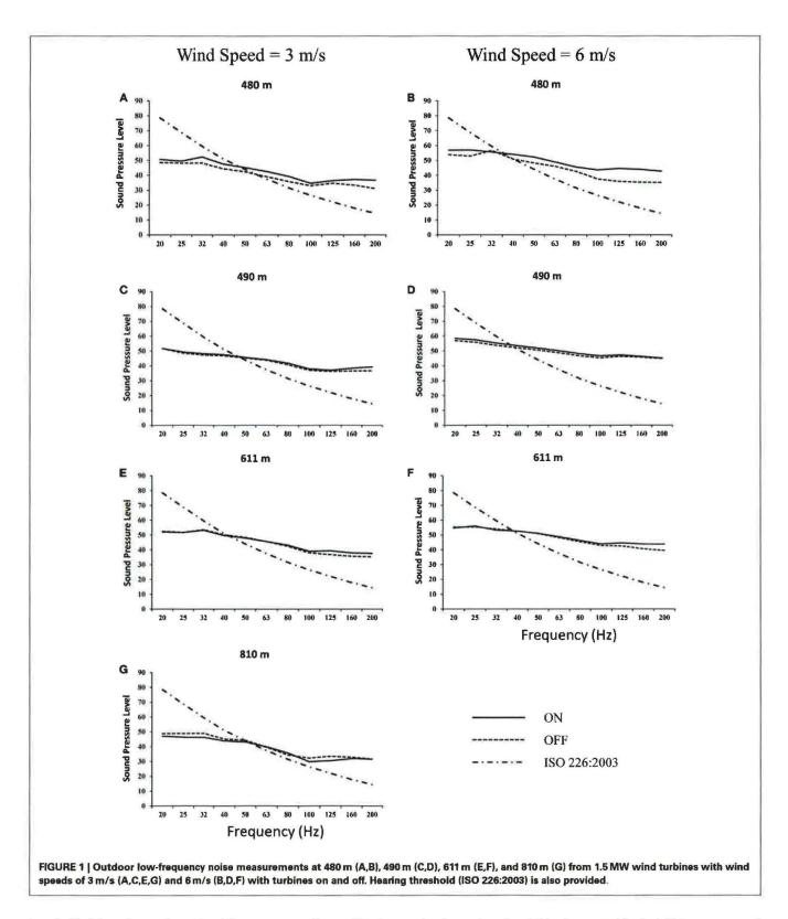
least half of that observed at 480 m. The mean overall sound levels reported in dB(A) showed very similar trends to those reported in the LFN analysis. Critically, the increase in mean sound levels at the closest location (480 m) reported in the LFN spectrum and overall sound in the 1/3-octave band analysis was maintained. In addition, the observed trends at 490, 611, and 810 m, also remained
