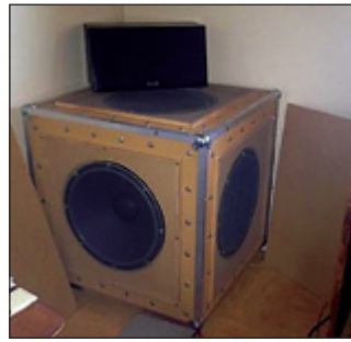
Figure 10. Loudspeakers for WTIS synthesis in 43 m 3 test room.
