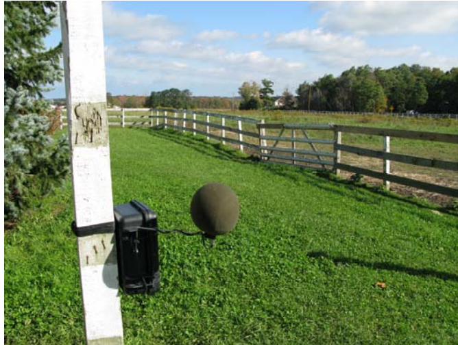
Figure 4.3.3.2 Typical Integrating Sound Monitor with 7" Weather-treated Windscreen
