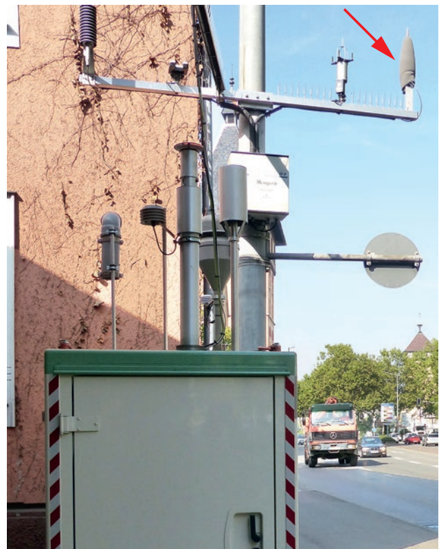
Figure 5.2-2: LUBW measuring station for detecting road traffic noise in Reutlingen, Lederstrasse. The arrow shows the location of the microphone. Photo: LUBW
