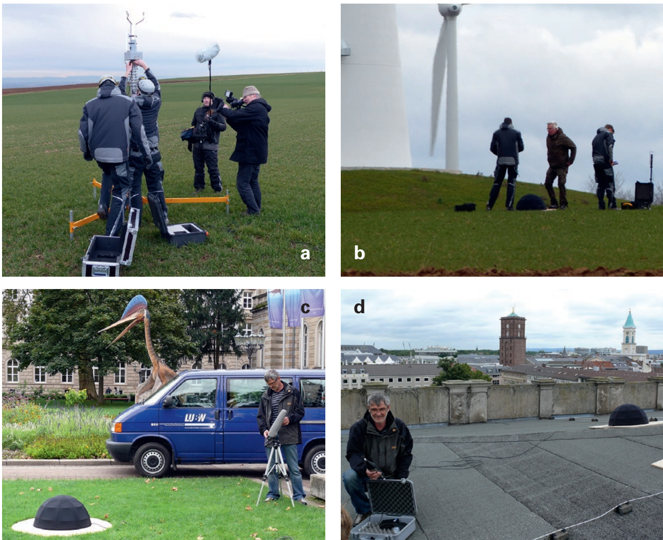
Figure 2-2: Impressions of the measurements during the execution of the measurement project. a) Construction of a wind measuring mast (top left) and b) of a measurement point (top right) during measurement at a wind turbine. c) and d) Setup of measurement points in the city centre of Karlsruhe (bottom). Photos: LUBW
