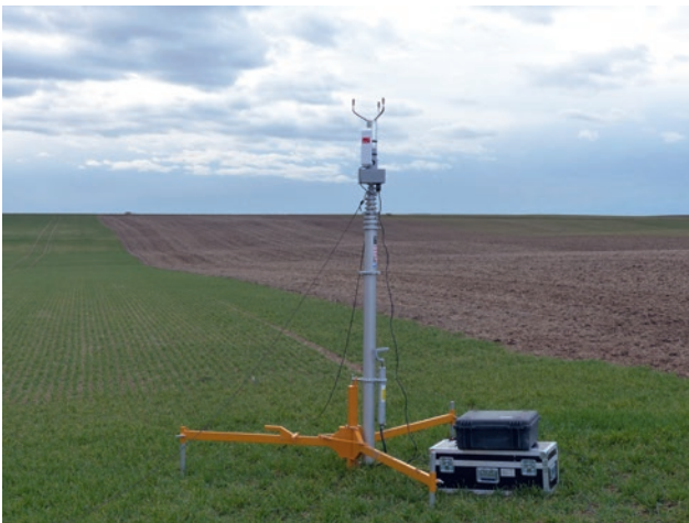
Figure 4.5-4: Anemometer mast for measuring wind speed and wind direction, air pressure, humidity and temperature. The mast is extended to 10 m (not yet extended in the image). Photo: LUBW
