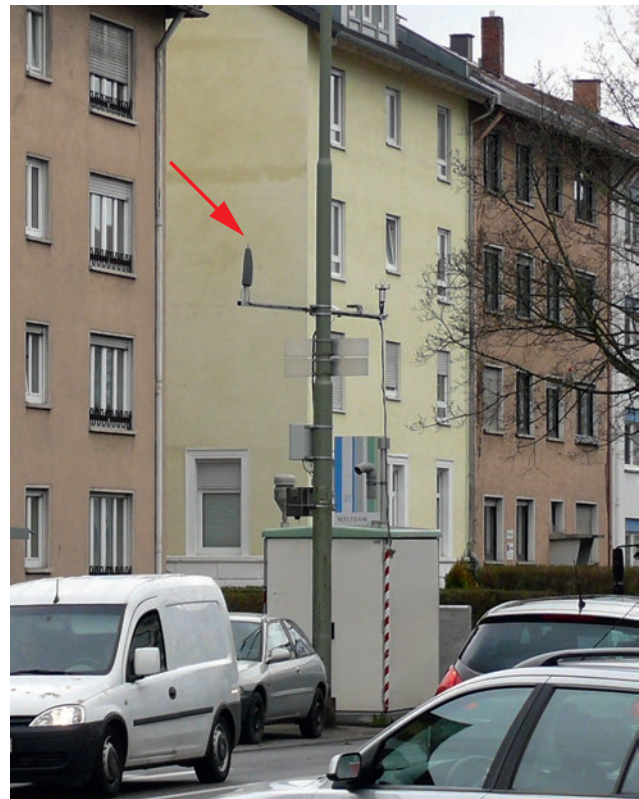
Figure 5.2-1: LUBW measuring station for detecting road traffic noise in Karlsruhe, Reinhold-Frank-Strasse. The arrow shows the location of the microphone. Residential buildings visible in the background. Photo: LUBW
