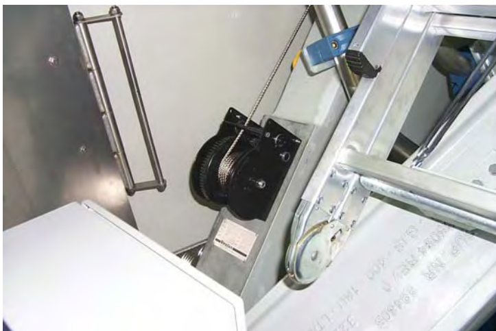
Figure 10 The Crane Winch placed on foundation.
