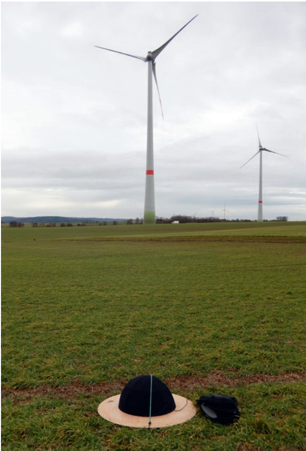
Figure 4.7-1: Wind turbine WT 6 in surroundings used for agricultural purposes. The measurement point MP1 with reverberant plate and dual wind screen can be seen in the foreground. Photo: Wölfel company
