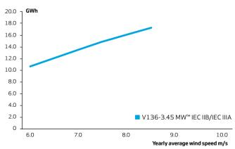
One wind turbine, 100% availability, 0% losses, k factor =2, Standard air density = 1.225, wind speed at hub height
