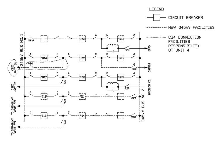
CBEC 345kV SUBSTATION CONCEPTUAL ONE-LINE DIAGRAM
