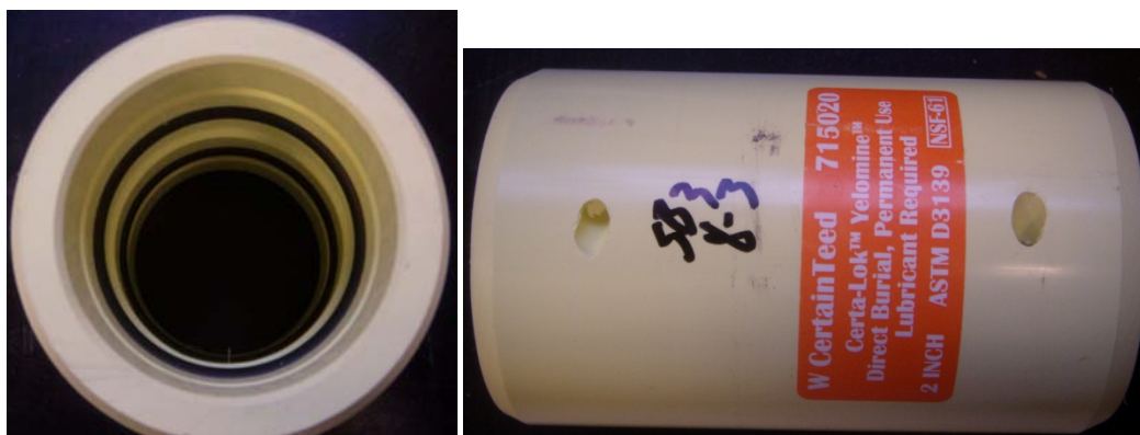
Figure 3.6. A joint coupling with Polyisoprene gaskets (permanent coupling).
