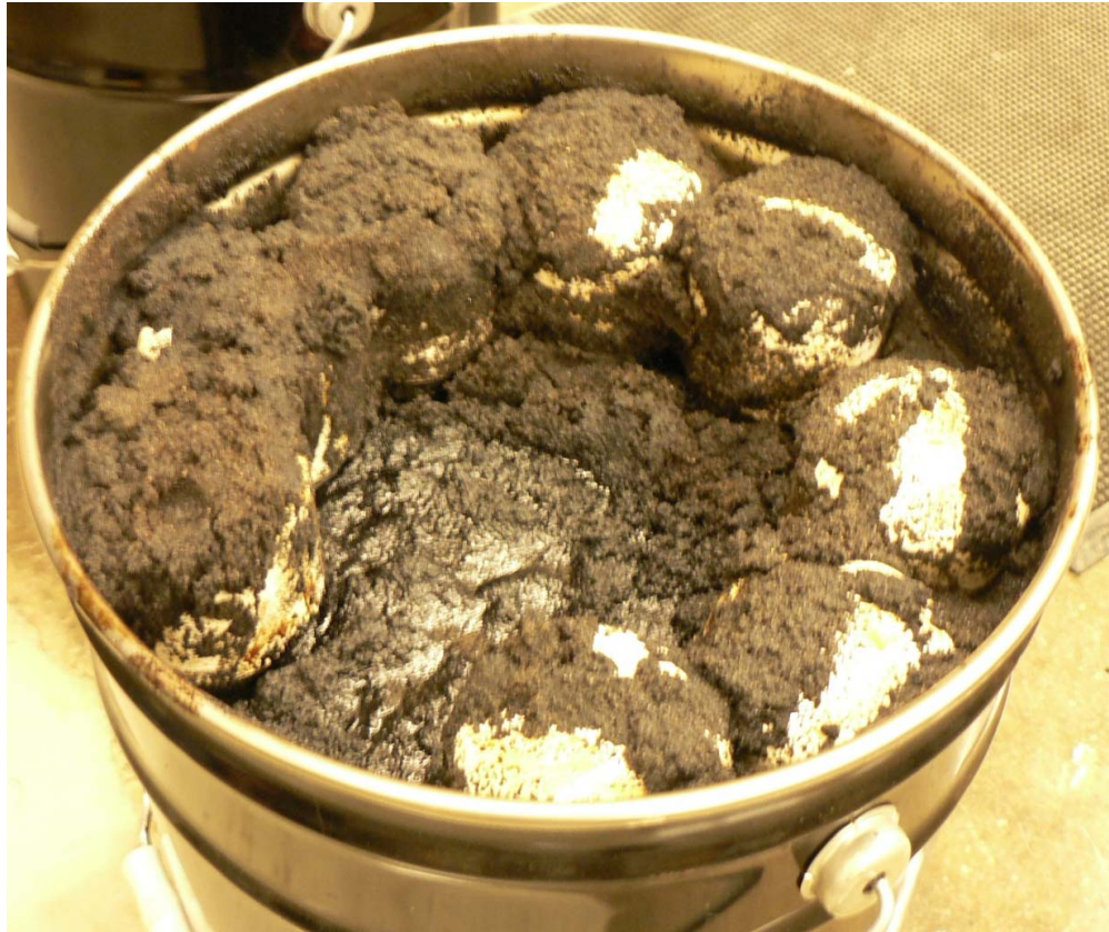
Figure 3.8. 10.5 inch pipe specimens immersed in sand and Oil-C.
