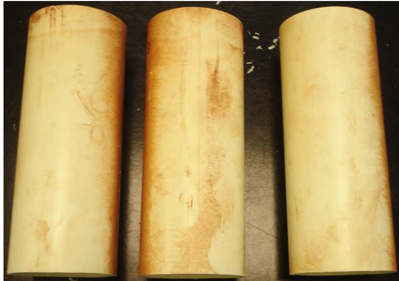
Figure 3.9. Six-inch pipe specimens used in the parallel plate compression test.
