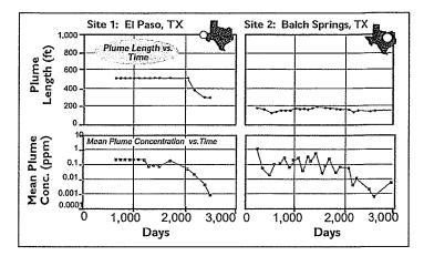
Plume Concentration Trend: For each sampling episode, the average benzene concentration in the plume area was estimated using Delauney triangulation (Isaaks and Srivastava, 1989), an area-weighted averaging procedure involving subdivision of the plume area into triangular segments defined by adjacent wells. Average concentration vs. time was plotted for each site to define change over time.
